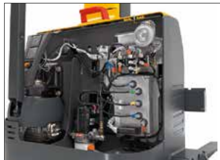
Sealed AC motor, controllers and connectors
